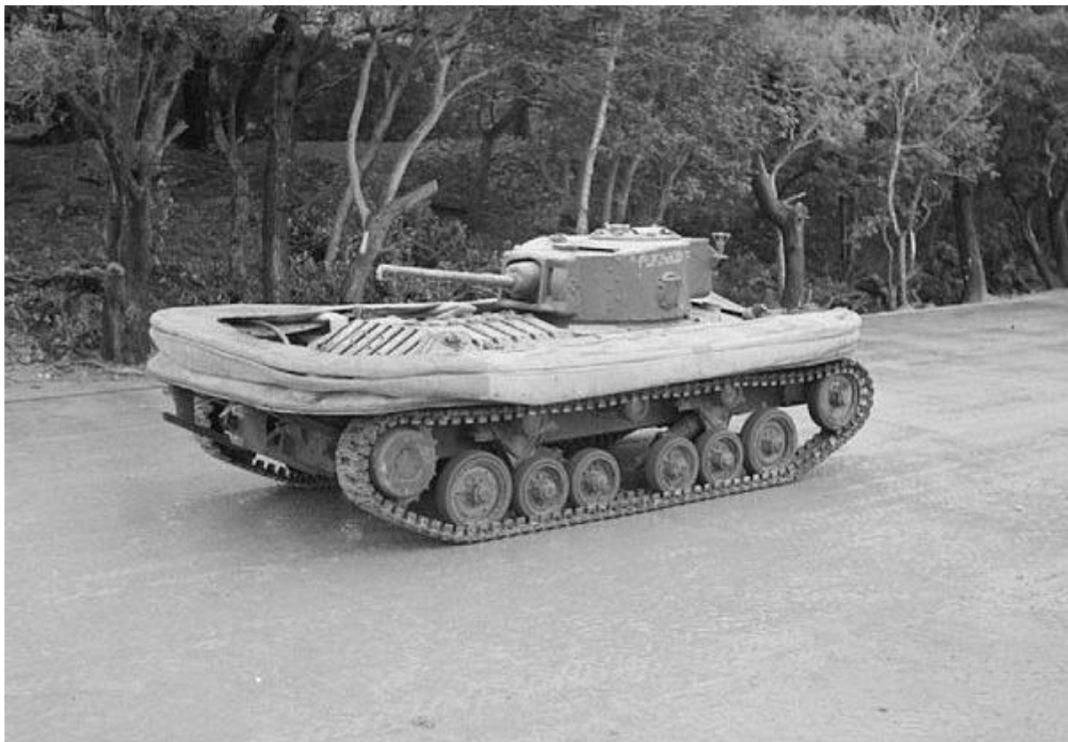
Valentine DD tank with screen lowered and gun pointing towards the rear of the vehicle.
